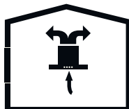
Fig. 6: Air Circulation with Carbon Filter
