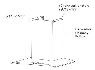
6. Carefully slide the decorative chimney top down inside the decorative chimney bottom. Raise the decorative chimney top until its holes align with holes in the chimney mounting bracket (located on the wall). Secure the chimney with 2 screws M4\*6mm.
