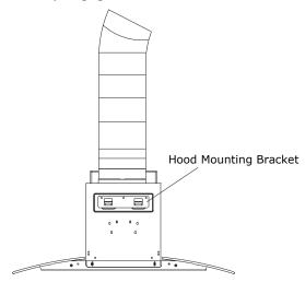
Carefully place the decorative chimney bottom into the recessed area of the hood body top. Secure the decorative chimney bottom to the wall using (2) ST 2.9 x 14mm mounting screws and dry wall anchors.
